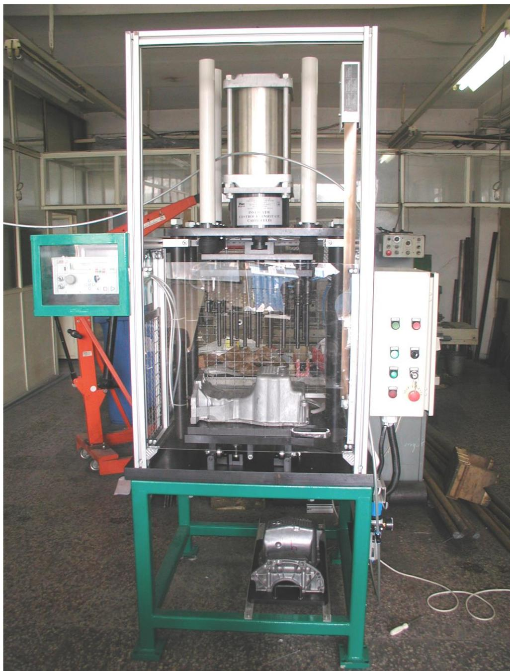
Instalație control etanșitate carter ulei | Tightness control equipment for oil pan
